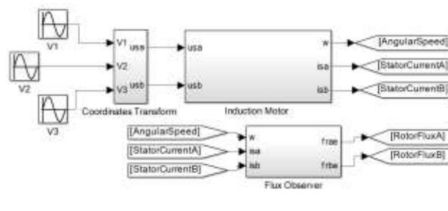
Figure 3 – Observer for the rotor flux.
