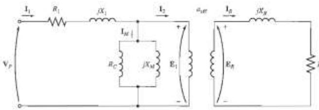
Figure 1 – Real Equivalent Circuit of Induction Motor.
