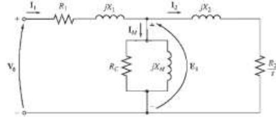
Figure 2 – Simplified Equivalent Circuit of Induction Motor.
